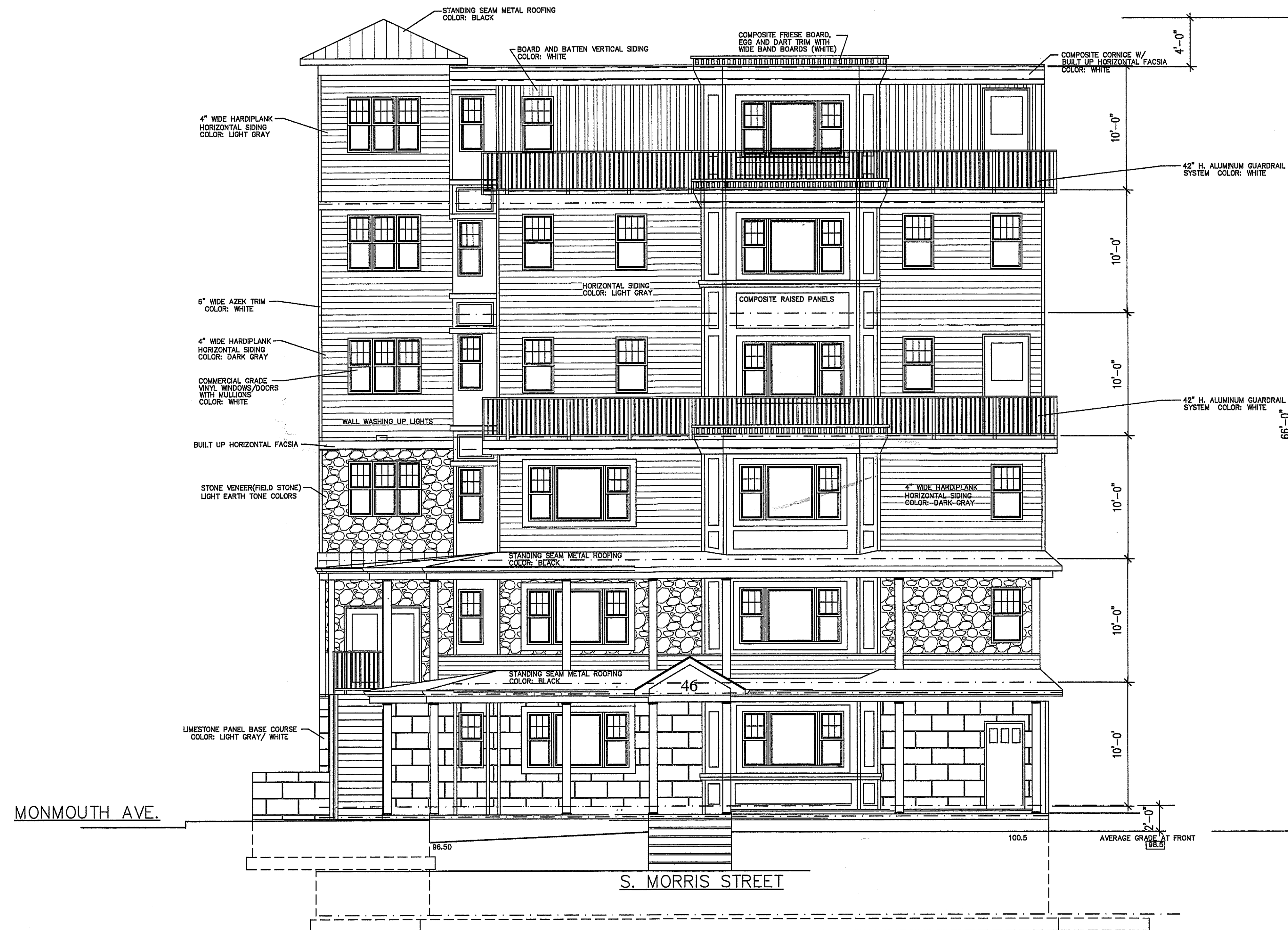
46 S. MORRIS ST.- FRONT ELEVATION-APARTMENTS SCALE: 3/16" = 1'-0"
