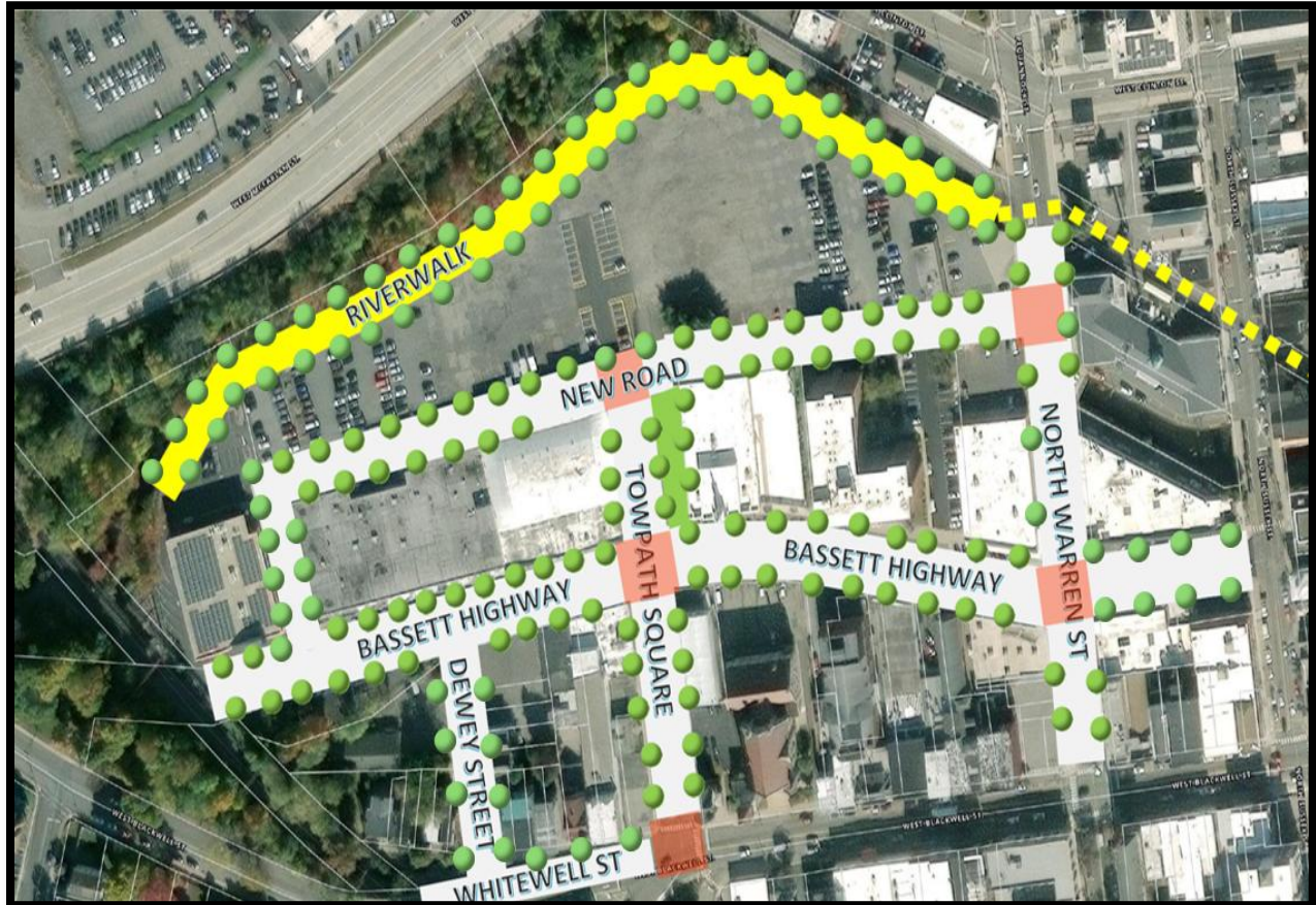
Figure 8 ~ Vehicle Circulation and Pedestrian Mobility Plan (the design intent is for tree-lined streets for those streets labelled above; for an extension of Towpath Square realigned as shown with green space adjacent as shown; and for a riverwalk along the Rockaway River as shown in yellow, connected to rails-to-trails conversion of the existing rail line as shown in dashed yellow; and decorative stamped concrete at key intersections as shown in red squares). See also Section 4.13.
