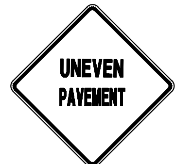
IF AND WHERE DIRECTED BY ENGINEER W8-9A 'UNEVEN PAVEMENT' 30" X 30" BLACK LETTERS ON ORANGE BACKGROUND
