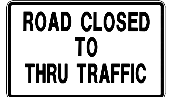
R11-4 'ROAD CLOSED TO THRU TRAFFIC' 60" X 30" BLACK LETTERS ON WHITE BACKGROUND
