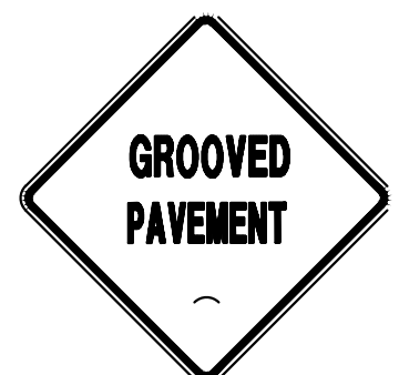
IF AND WHERE DIRECTED BY ENGINEER W8-14A 'GROOVED PAVEMENT' 30" X 30" BLACK LETTERS ON ORANGE BACKGROUND
